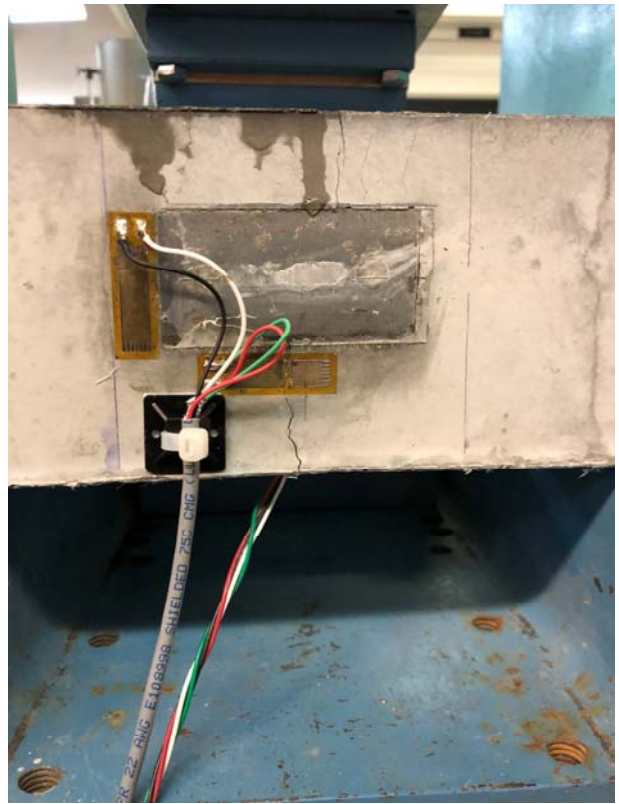
Four-point bending test with embedded wireless strain gauges
