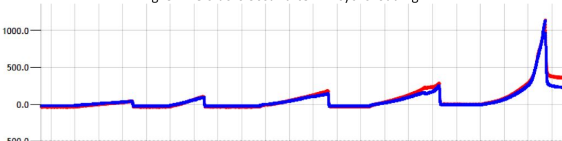
Fig. 4 Sensor system successfully detects strain up to 1000 \times 10^{-6}
