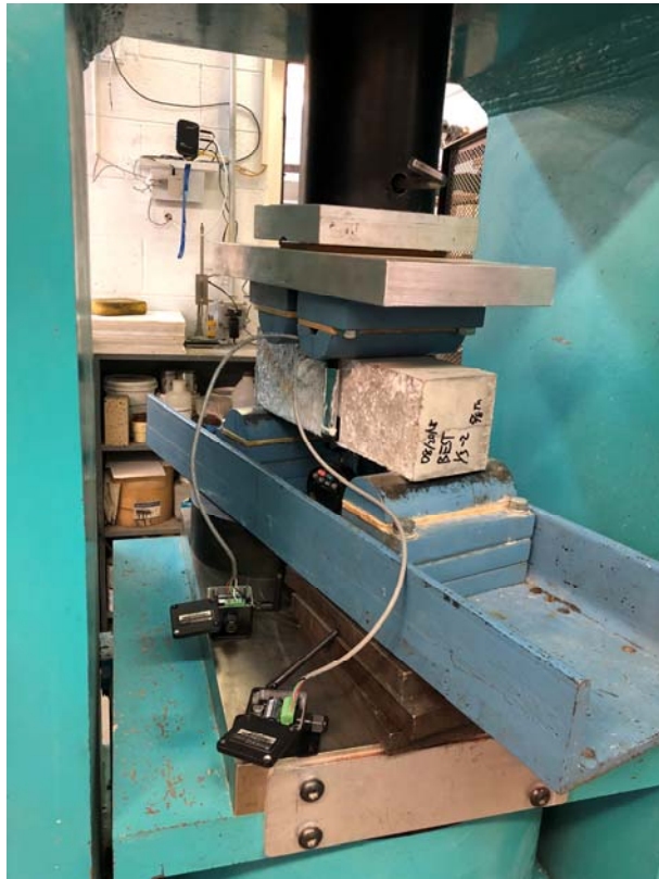
Four-point bending test with embedded wireless strain gauges
