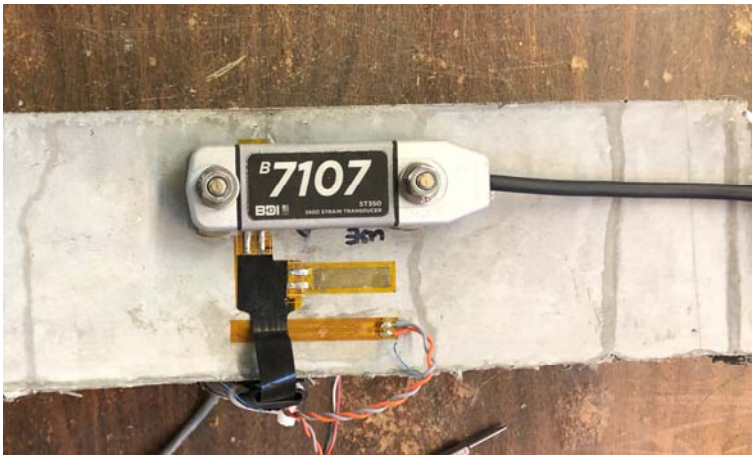
ECC prism with embedded strain gauges and BDI Strain Transducer
