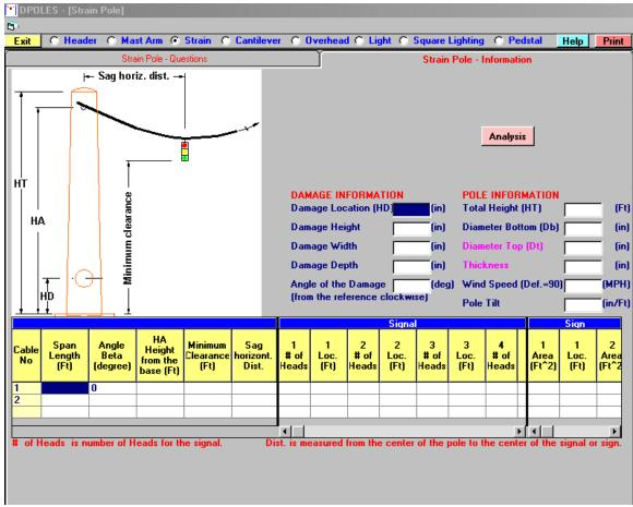
Figure 3.3 – Strain Pole Input Page
